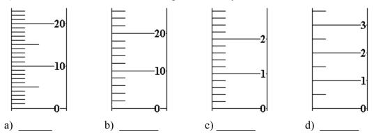
When reading a graduated cylinder you need to keep the graduated cylinder on the desk and lower your eyes to the level of the meniscus and you read where the bottom of the meniscus is. Be sure to include one point of estimation in your reading.
