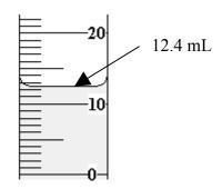
2) Determine the volume of the liquids in the following cylinders:
